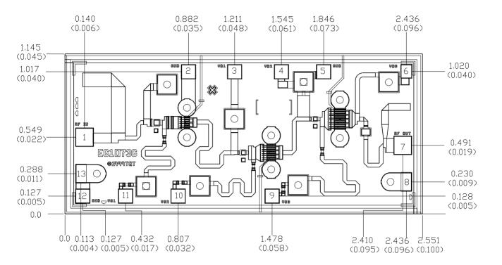
Units: millimeters (inches) Thickness: 0.1016 (0.004) Chip edge to bond pad dimensions are shown to center of bond pad Chip size tolerance: +/- 0.051 (0.002)
