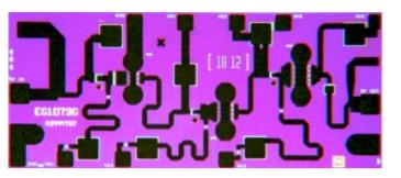
The TriQuint TGA1073G-SCC is a three stage MPA MMIC design using TriQuint's proven 0.25 um Power pHEMT process. The TGA1073G-SCC is designed to support a variety of millimeter wave applications including point-to-point digital radio and point-to-multipoint communications.
